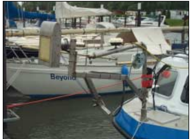
Figure 6: Mount of the transducer at a survey boat
