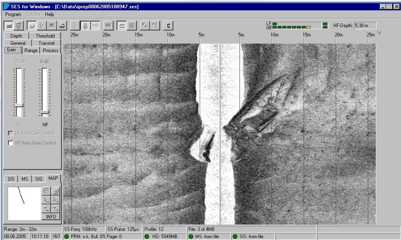
Echo plot sample of the SES-2000 Side Scan Extension from the river Elbe (wreck located on the river bed and partly buried within the sand, water depth around 5m, small sand ripples at port side) System parameters: frequency 100kHz, pulse length 125µs, operating range 2m - 32m
