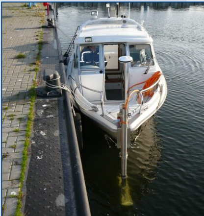
Transducer mounted on a survey vessel
